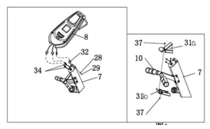
**Step 8:** Fix the lock Vertical tube cover (38 L/R) to the Vertical tube (7) with Screws (26).
