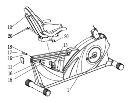
Note: The TIGHTNESS between the Seat Assembly and the Rail can be adjusted via adjusting the Eccentric Axle of the Wheel. Both sides can be adjusted.
