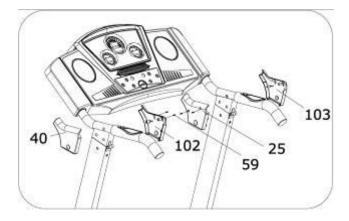
With ST4.2\*12 Screw(59),Insert the UPRIGHT COVER(25,103,40,102) onto the L&R handle bar.
