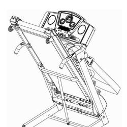
Support place A with hand, then pull up following the arrow direction, till hearing the sound that the cylinder B is locked into the round tube
