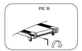
Picture A If the belts has drifted to the RIGHTPicture BIf the belts has drifted to the LEFTWARNING: ALWAYS UNPLUG THE TREADMILL FROM THE ELECTRICAL OUTLET BEFORECLEANING OR SERVICING THE UNIT.
