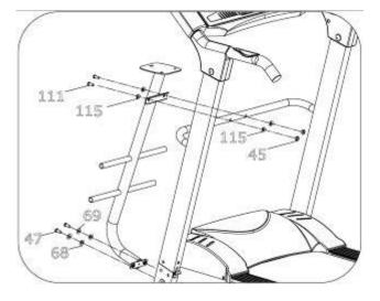
1.Use 5# Allen Wrench , drill the bolt M8\*25(47) through the flat washer 8 (69), spring washer 8 (69), then lock the supporting frame (94) onto the main frame (1);
