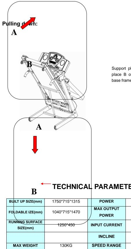
Support place A with hand , kick the place B of air pressure bar, then the base frame will fall down automaticlly
