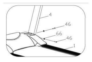
Use the 5# allen wrench, drill through the bolt (46) to Lock washer(66), then lock the Right upright (4) onto MAIN FRAME (1)
