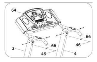
Use the 5# allen wrench, drill through the bolt (46) to Lock washer(66), then lock the COMPUTER (64) onto R&L upright (3,4).
