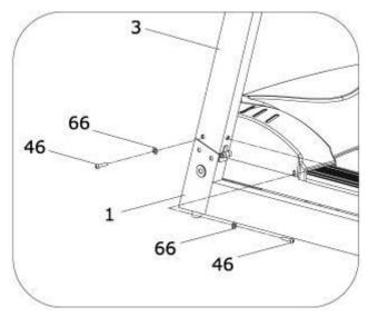
Use the 5# allen wrench, drill through the bolt (46) to Lock washer(66), then lock the Left upright (3) onto MAIN FRAME (1)
