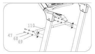
Use 5# Allen Wrench, drill the Bolt(47) M8\*25 through the flat washer 8(69), spring washer 8(69), then lock the connecting frame(110) onto the left and right upright(3,4)
