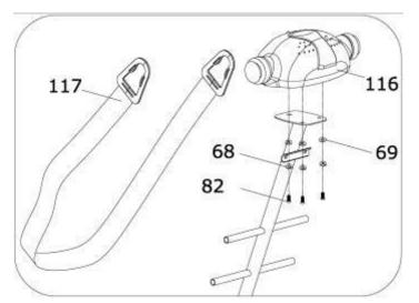
1. Use 5# Allen Wrench, drill Bolt M8\*15 (82) through the spring washer (68), flat washer (69), lock the massage head (116) onto the supporting frame (112)
