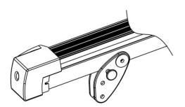
As above drawing, you can adjust lifting angle by changing pin's position. There are 3 sections adjust key to be used.
