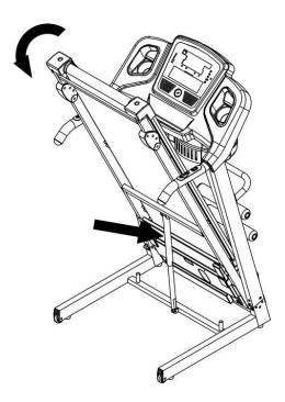
Kick the safety sleeve lightly and pull down the machine at the same time as the arrow direction. Then the machine will fall down smoothly.
