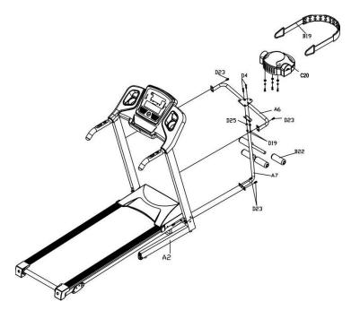
Step 4: Put on the SAFETY KEY (C14) and Mp3 line (C19)
