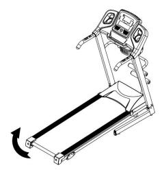
Lift up the machine and force to pull up until you heard "click" that made by safety casing stuck the pneumatic cylinder.
