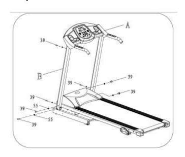
Fix the upright tube(B) and console tube(A) to the main frame with M8\*15 allen (39) and washer (55) by using 5# Allen wrench(12).
