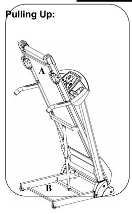
Put your hand on A position, then lift up the base frame till hearing the sound that the air pressure bar B is locked into the tube.
