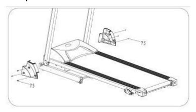
Fix the Left & Right Upright Tube Cover(33,34) to the base frame with bolt M5\*12(75) by using Wrench w/ screw driver.
