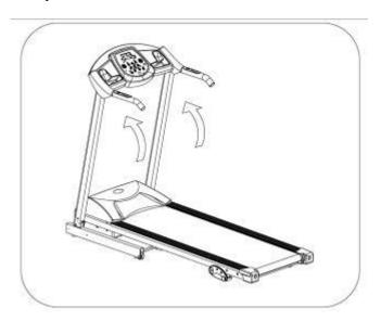
Lift up the Computer A and Upright tube B with the arrow direction.
