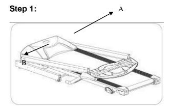
Open the carton, get out the above spare parts, and put the Main Frame on the level ground.
