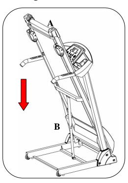
Support place A with one hand, then kick the air pressure bar at the position B, press the base frame, then it will fall down automatically ( Please keep anybody and any pet away the machine when it is falling down)
