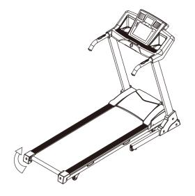
Lift up the machine and force to pull up until you heard "click" that made by safety casing stuck the pneumatic cylinder.
