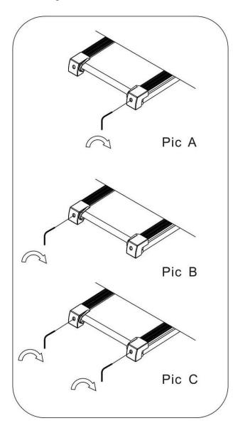
If the belt has drifted to the right, unplug the safety lock and power switch, and turn the right adjusting bolt 1/4 turn clockwise, then insert the power switch and safety lock, make the treadmill running, observe the running belt deviate condition. Repeat above steps until the running belt be placed in the middle. **See**
