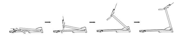
STEP 2: According to the picture to tight the bolt M8\*15 (D2) and inner washer (D20)
