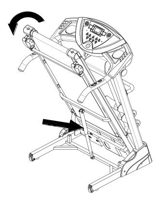
Use foot to kick the safety sleeve lightly and pull down the machine at the same time as the arrow direction. Then the machine will fall down smoothly.
