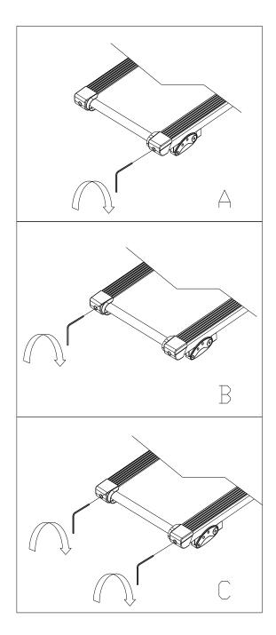
Place treadmill on a level surface. Make treadmill run at approximately 6-8 km/h, observe the running belt deviate condition.
