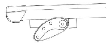
Adjust the incline by moving the pin, There are three levels.
