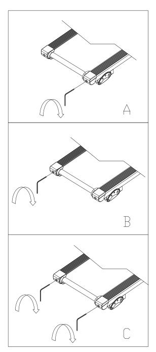
If the belt has drifted to the right, unplug the safety lock and power switch, and turn the right adjusting bolt 1/4 turn clockwise, then insert the power switch and safety lock, make the treadmill running, observe the running belt deviate condition. Repeat above steps until the running belt be placed in the middle.
