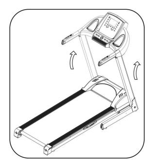
1.Open the carton, get out the above spare parts, and put the Main Frame onto the level ground.
