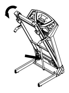
Kick the safety sleeve lightly and pull down the machine at the same time as the arrow direction. Then the machine will fall down smoothly.
