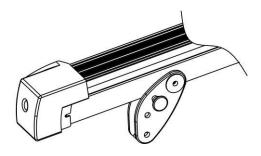
As above drawing, you can adjust lifting angle by changing pin's position. There are 3 sections adjust key to be used.
